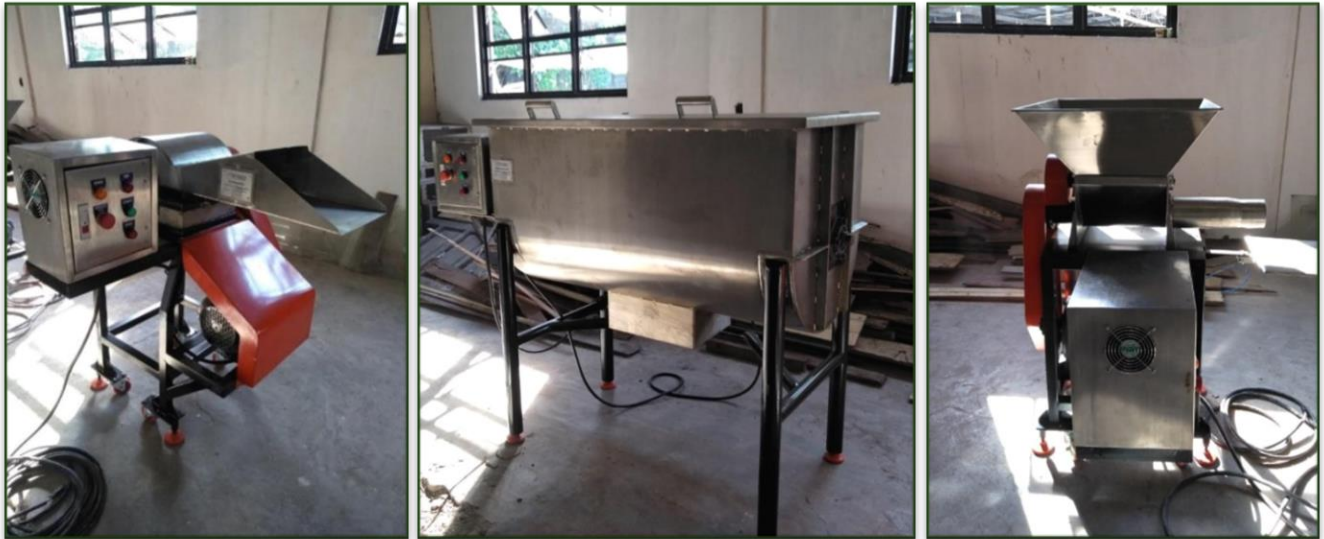
Figure 28. BPI rice straw chopper (left), BPI mushroom substrate bag filler (middle) and BPI mushroom substrate mixer (right).
