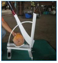
Three male workers were assigned to perform slicing of squash fruit using the tool and a kitchen knife. Each worker was given 10 pieces of squash fruits, weighing two kilograms each. The average time (in minutes) in slicing the fruit using the tool and manual processing was determined. The average number of squash fruit processed per day was also recorded.
